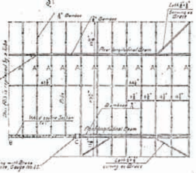
SECTION OF ASSEMBLY C OF THE WING OF WOOD WITH THE 2 BAMBOO PICES
