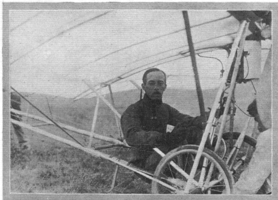
In the above central view of the "Demoiselle" M. Santos Dumont is occupying the somewhat rough and ready canvas seat that is provided for the pilot. He has in his right hand the elevating lever, which moves the universally-jointed tail up or down; his left hand is grasping the small wheel which serves to steer the machine by moving the rudder sideways, and at his back is the lever that enables him to flex the wings by leaning his body over to one side or the other.
